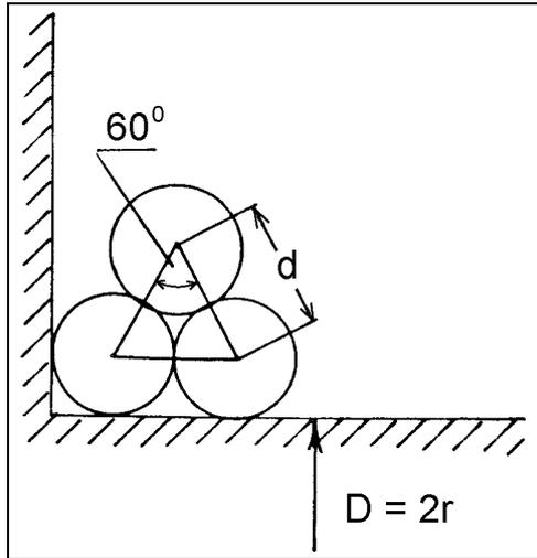
Fig. 3. Scheme of rope reeling on the drum.
