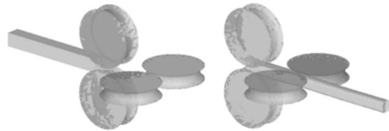
Fig.2. Simulation of rolling in a roughing train of a wire rod mill.
