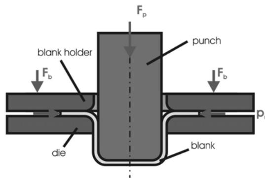
Fig.4. Schematic draft of deep drawing supported by radial pressure.
