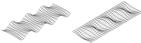
Fig.3. Edge and centre waves of a sheet.
