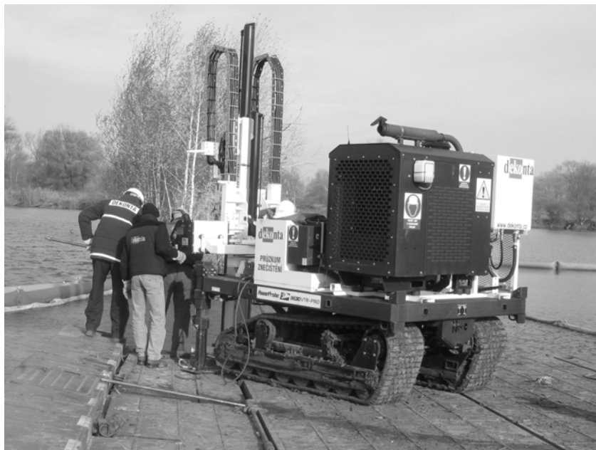
Obr. 2. Multifunkčná vrtná súprava AMS Power Probe 9630 VTR-PRO Fig. 2. AMS Power Probe 9630 VTR-PRO multifunctional drilling rig
