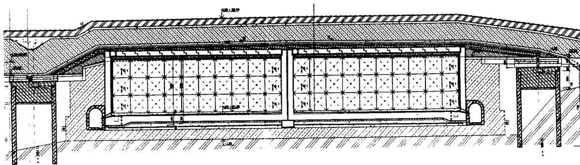
Fig. 2. Schematic cross section of the twins of underground chambers in a definitive container's storage position.
