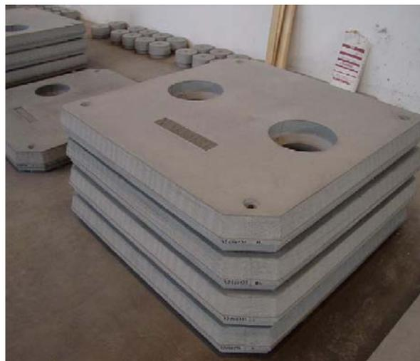
Fig. 6. Precast container body and cover plates made of HPFRC.
