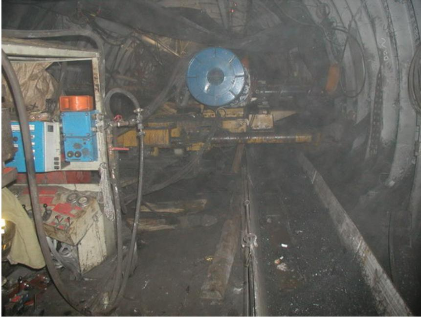
*Fig. 4. Drilling part of the system at the borehole mouth.*
