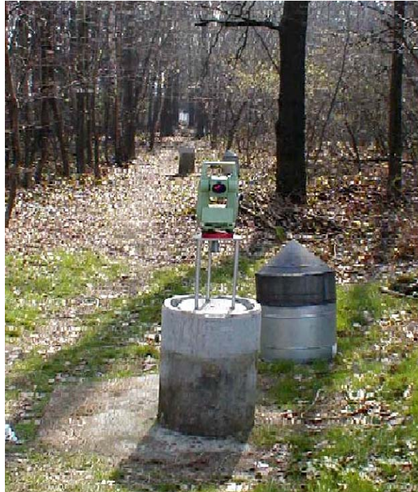
Fig. 1. IGDM rangefinder base in Ostrava – Krasne Pole.
