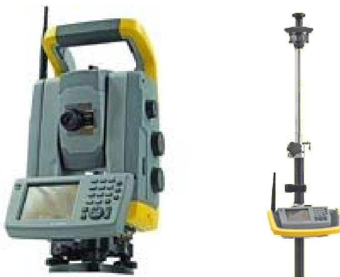
Fig. 3. Trimble S6 Robotic, a range pole with an omnidirectional prism.
