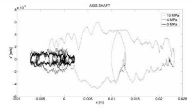
Fig. 3. Phase trajectories runs estimated from vibrations signal measured on axis shaft.
