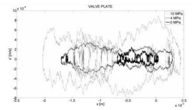
Fig. 5. Phase trajectories runs estimated from vibrations signal measured on valve plate.
