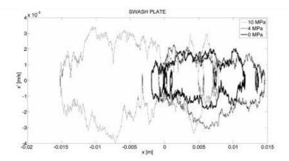
Fig. 6. Phase trajectories runs estimated from vibrations signal measured on swash plate
