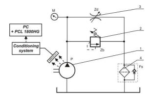
Fig. 1. Simplified diagram of the laboratory station.
