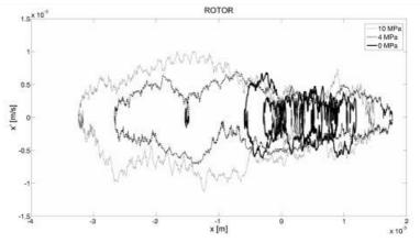
Fig. 4. Phase trajectories runs estimated from vibrations signal measured on rotor.
