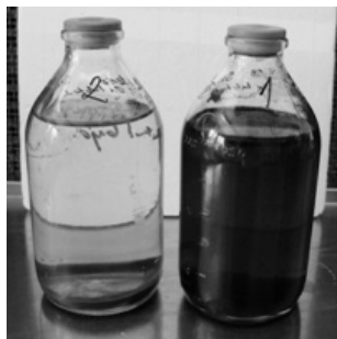
Fig. 2. Reaction flask during SRB cultivation; flask 1- with black precipitates of iron sulphides; flask 2 - without visible iron sulphide precipitates.
