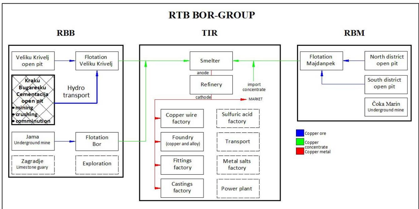
Fig. 5. Process of mining, processing and refining at the site Kraku Bugaresku - Cementacija within RTB Bor Group.
