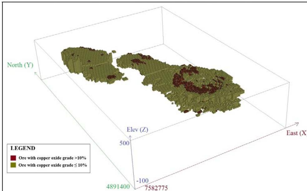
Fig. 4. Block model of a copper deposit Kraku Bugaresku – Cementacija.
