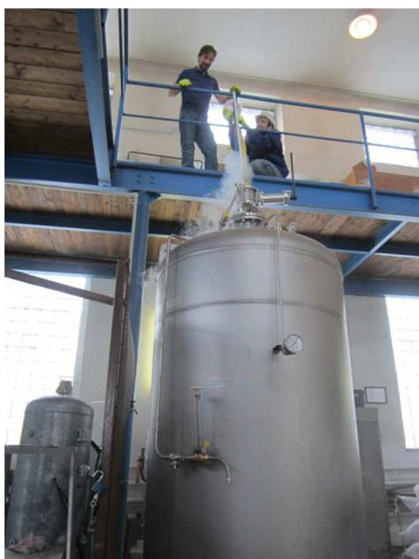
Fig. 1. Filling of the VAZEP device with powder zeolite (fraction: 0,1 – 1 mm).
