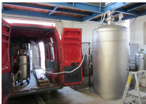
Fig. 2. First-stage cooling (77 °K).
