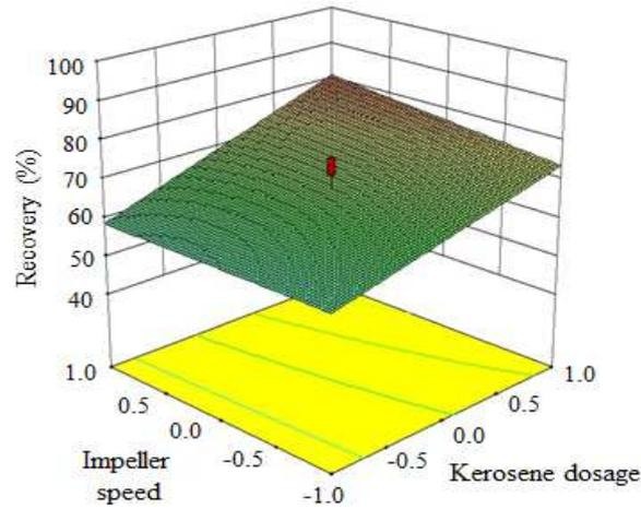
Fig. 6. 3D variation of recovery with respect to impeller speed and kerosene.
