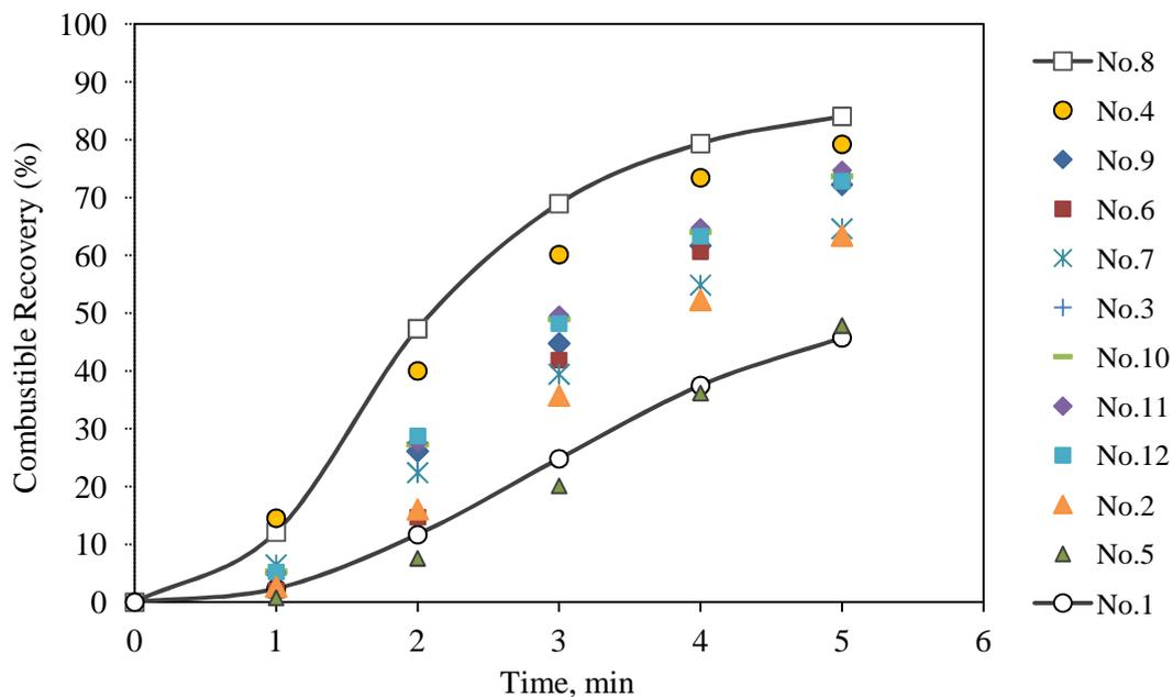
Fig. 1. Flotation recovery of combustible matter as a function of time.
