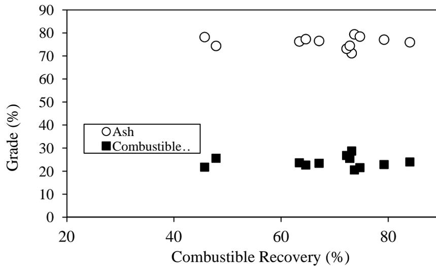
Fig. 2. Concentrate grade as a function of recovery.
