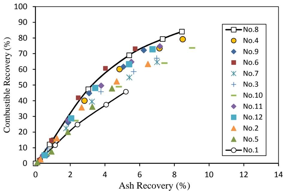
Fig. 3. Recovery of combustible matter versus recovery of ash.
