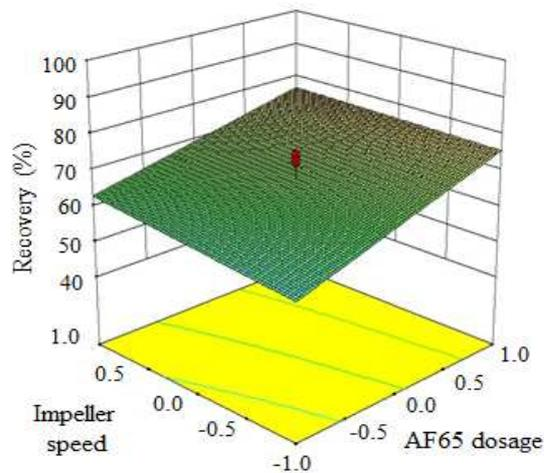
Fig. 5. 3D variation of recovery with respect to impeller speed and frother dosage.
