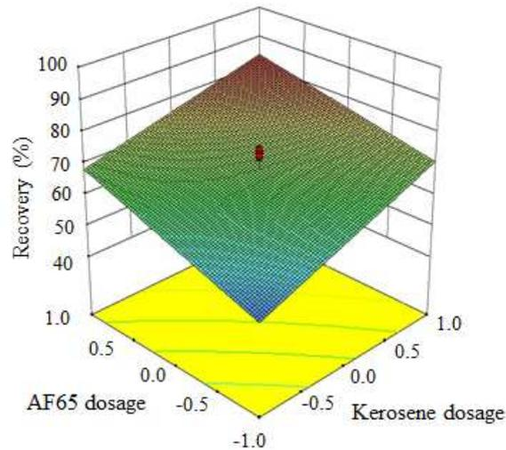
Fig. 4. 3D variation of combustible recovery with respect to frother and collector dosage.
