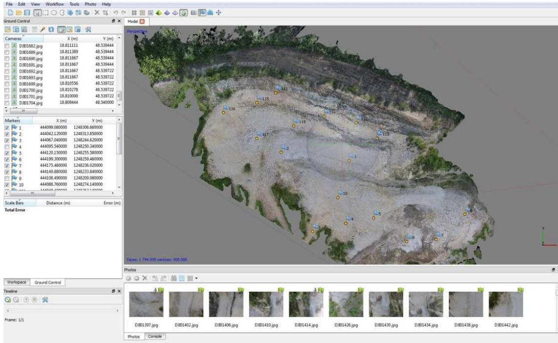
Fig. 5. Image processing in Agisoft PhotoScan software – result of the processing as a textured point cloud.
