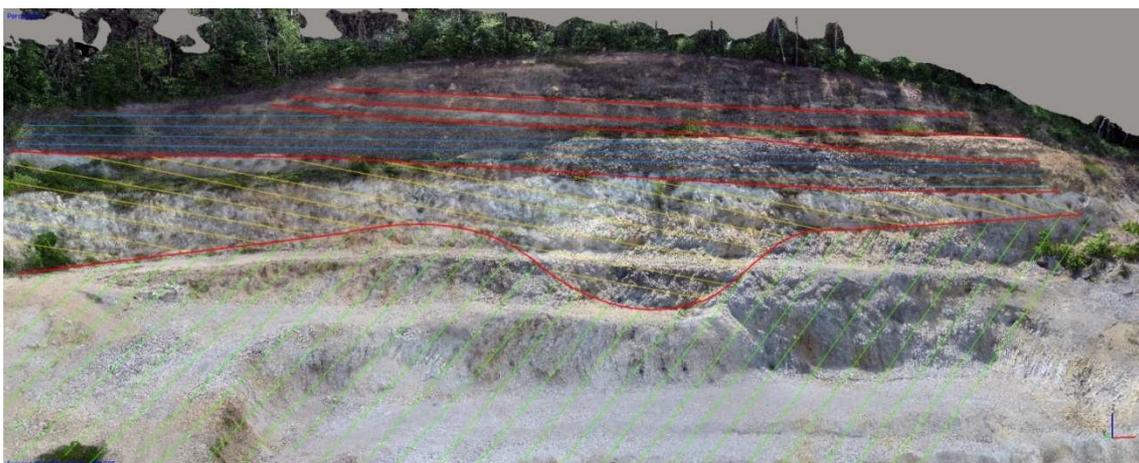
Fig. 6. Geological structure interpreted on the basis of the photo plan.
