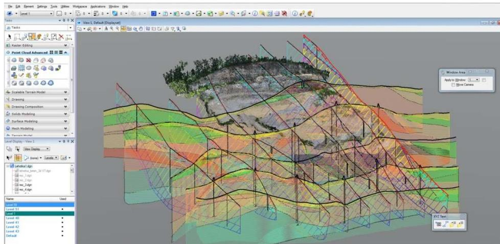
Fig. 7. Comparison of point cloud inserted into the CAD software and historical model of the geological structure with current state obtained photogrammetrically.
