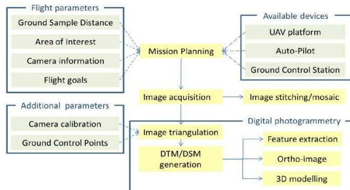
Fig. 4. Workflow for UAV data acquisition and processing (Nex and Remondino, 2013).
