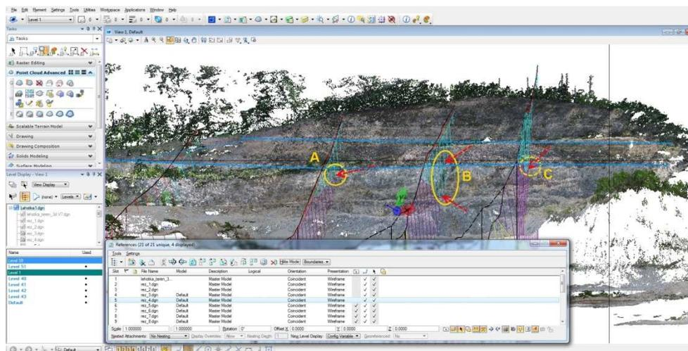
Fig. 8. Correlation of the models of the geological structure of the mineral deposit.
