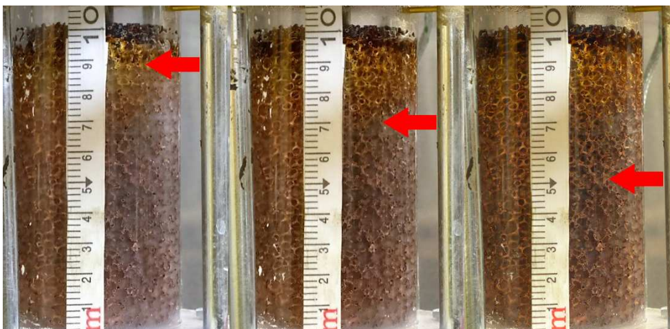
Fig. 8. Time-lapse image of phase change in heat storage unit (red arrow points to level between solid and liquid phase).
