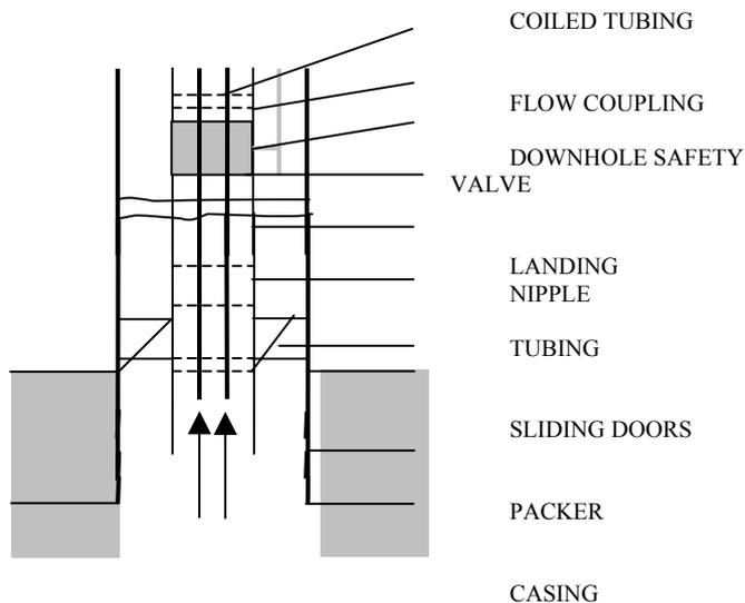
Fig 1. Coiled tubing as a velocity string
