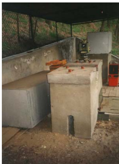
Obr. 1a. Stabilizačné zariadenie pre Väisäläho interferometer Fig. 1a. Stability equipment for Väisälä interferometer
