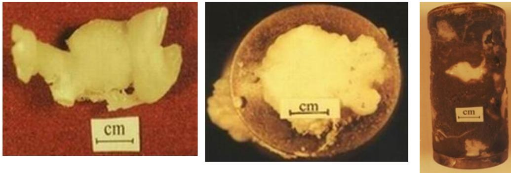
Fig. 2. A sample of natural hydrates from superficial «hydrates caps» (left and central) and a core from gas hydrates breeds with a mortar structure (right).
