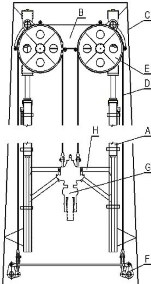
Fig. 1. The main elements of the RamRig<sup>®</sup> hoist assembly, showing the yoke (A), dolly (B), top drive (C), equalizer assembly (D), lifting wires (E) and the ramcylinders (F)
