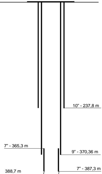
Fig. 2. Scheme of design of well LIPA 80.
