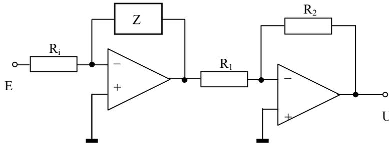
Fig. 1. Diagram of the electronic realization of the fractional-order operator.
