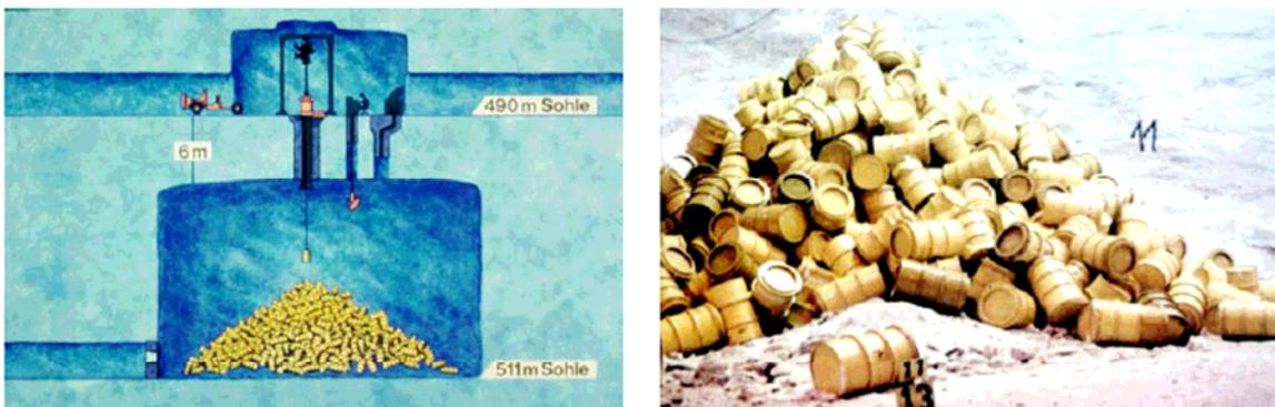
a) Lowering of ILW drums into the storage room      a) Unloaded ILW drums in the sealed storage room
