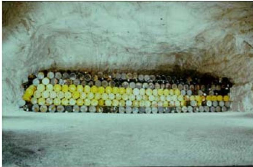
Fig. 2. Stacking technique for LLW drums in a mining chamber at the Asse mine (source GSF).
