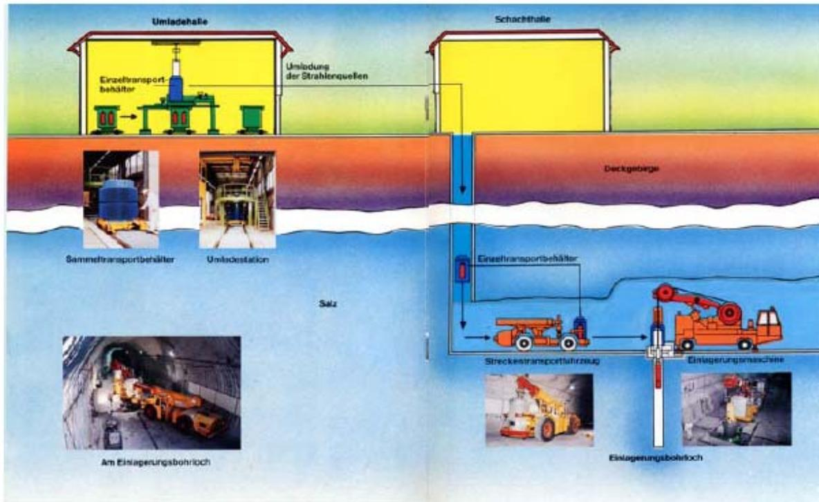
Fig. 5. Transport and handling system for HLW canisters developed and tested at the Asse mine.
