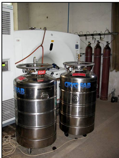
Fig. 13. Calculated MRI device with liquid helium dewars.
