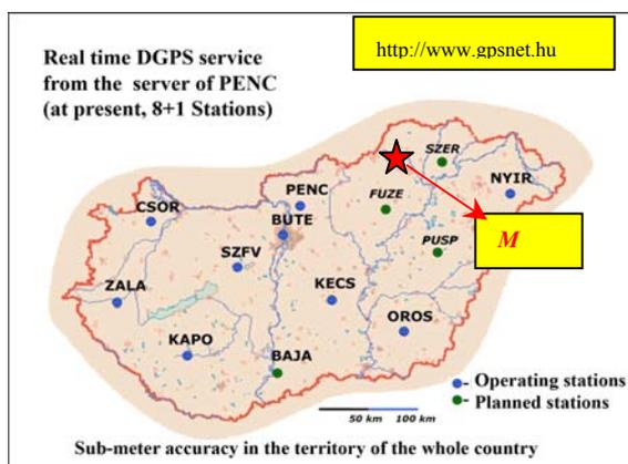
Fig. 1. The distribution of active GPS network.
