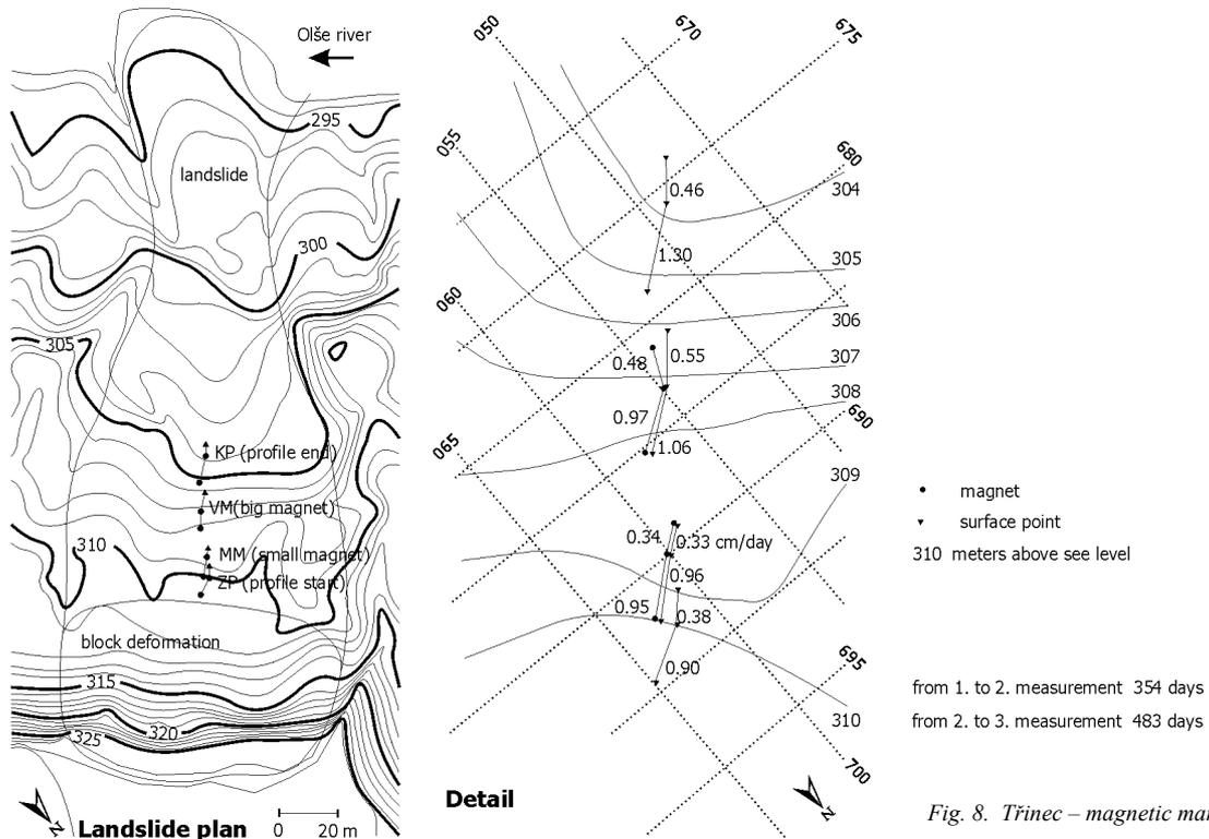
Fig. 8. Trinec – magnetic marks.
