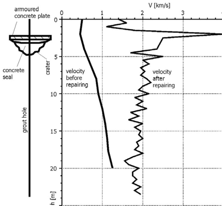
Fig. 4. Příbram – repeated velocity logging (modified by Bárta, 1996 a, b).
