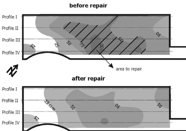
Fig. 7. Ostrava – repeated geoelectrical measurements.
