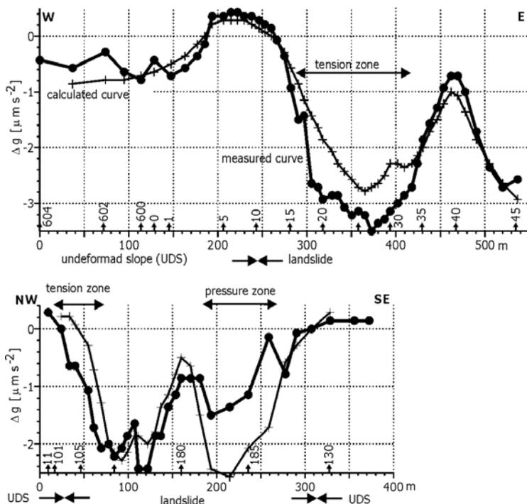
Fig. 5. Gravimetric measurements on landslide (modified by Calcagnile, et al., 1982).
