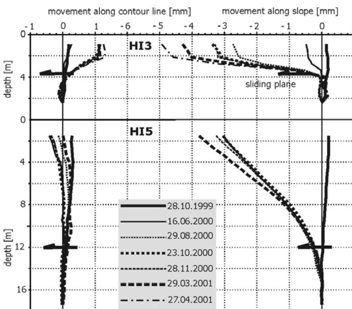
Fig. 1. Orlová-acurrate inclinometry (modified by Novosad, 2001).
