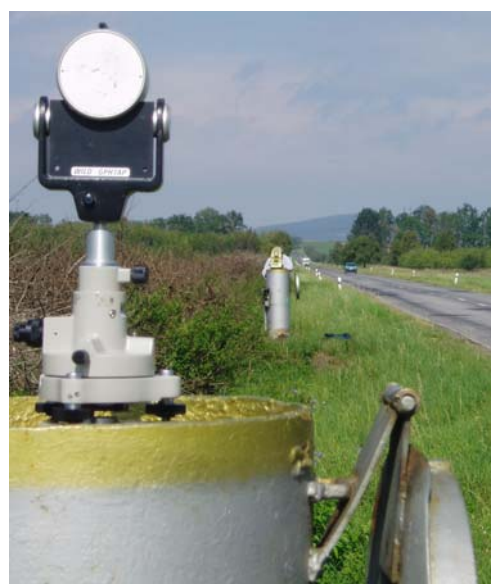
Fig. 3. Czech national long distances measuring standard - measuring with TS.
