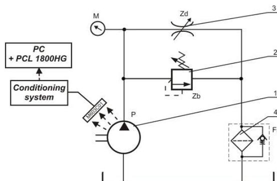
Fig. 1. Simplified diagram of the laboratory station.
