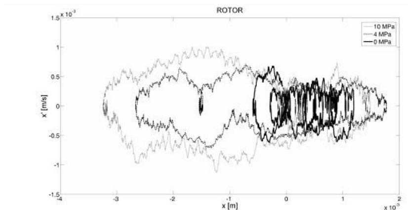
Fig. 4. Phase trajectories runs estimated from vibrations signal measured on rotor.
