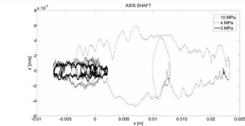
Fig. 3. Phase trajectories runs estimated from vibrations signal measured on axis shaft.
