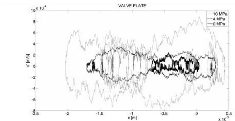
Fig. 5. Phase trajectories runs estimated from vibrations signal measured on valve plate.
