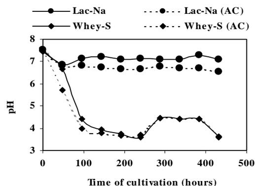
Fig. 13. pH values changes during the SRB cultivation. Substrate: solid whey – Whey-S; abiotic control – Whey-S (AC)
