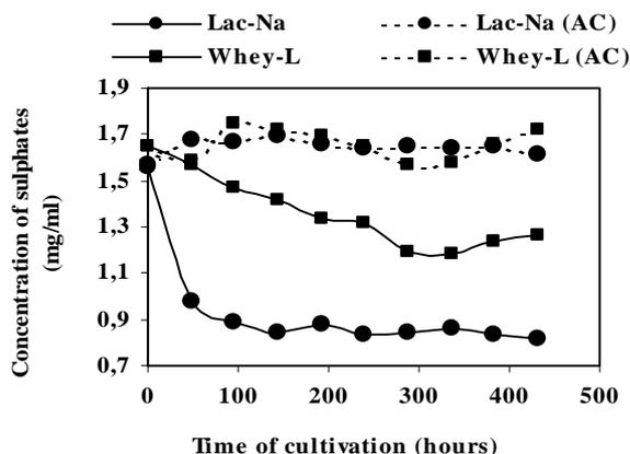
Fig. 10. Sulphate concentration changes during the SRB cultivation. Substrate: liquid whey – Whey-L; abiotic control – Whey-L (AC)
