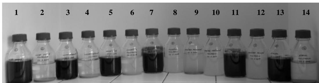
Fig. 1. Comparison of black precipitates formation during SRB cultivation using chosen substrates and abiotic controls (1) – sodium lactate; (2) – sodium lactate abiotic control; (3) – calcium lactate; (4) – calcium lactate abiotic control; (5) – saccharose; (6) – saccharose abiotic control; (7) – glucose; (8) – glucose abiotic control; (9) – solid whey; (10) – solid whey abiotic control; (11) – liquid whey; (12) – liquid whey abiotic control; (13) – ethanol; (14) – ethanol abiotic control.
