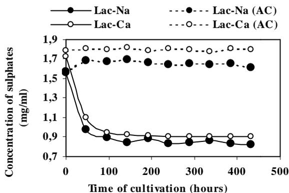
Fig. 2. Sulphate concentration changes during the SRB cultivation. Substrate: calcium lactate – Lac-Ca; abiotic control – Lac-Ca (AC)
