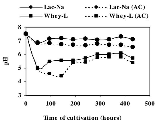
Fig. 11. pH values changes during the SRB cultivation. Substrate: liquid whey – Whey-L; abiotic control – Whey-L (AC)
