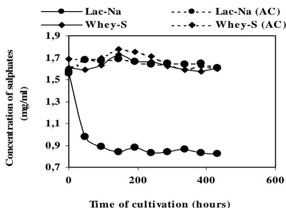
Fig. 12. Sulphate concentration changes during the SRB cultivation. Substrate: solid whey – Whey-S; abiotic control – Whey-S (AC)
