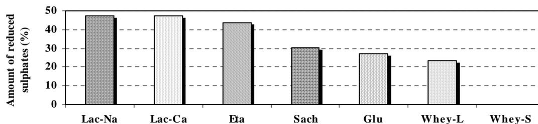
Fig. 14. Comparison of reduced sulphates amount by SRB using substrates: sodium lactate (Lac-Na), calcium lactate (Lac-Ca), ethanol (Eta), saccharose (Sach), glucose (Glu), liquid whey (Whey-L) and solid whey (Whey-S).
