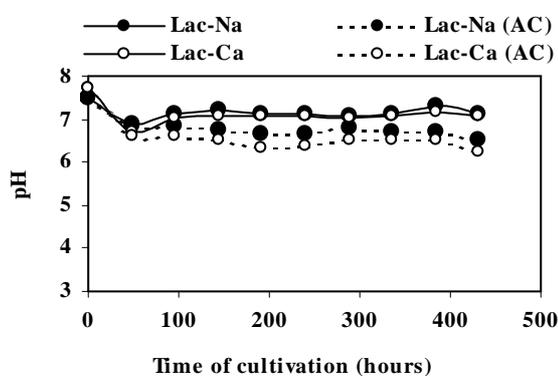
Fig. 3. pH values changes during the SRB cultivation. Substrate: calcium lactate – Lac-Ca; abiotic control – Lac-Ca (AC)
