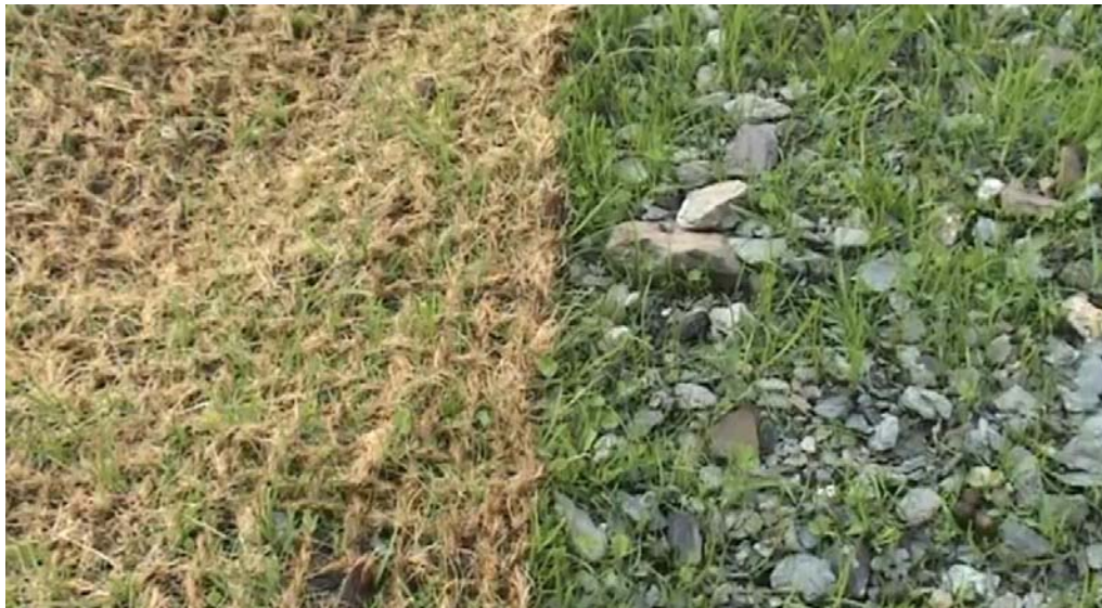
Fig. 7. Results of hydroseeding after about 2 months [1].
