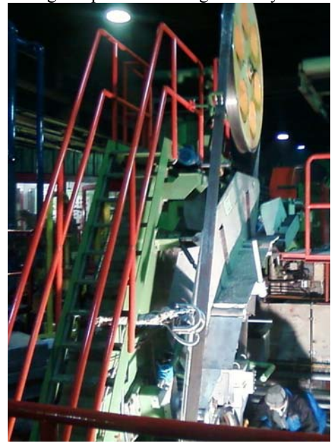
Fig. 2. Adjusted machinery equipment (part of the casting machine for continuous casting of copper)
