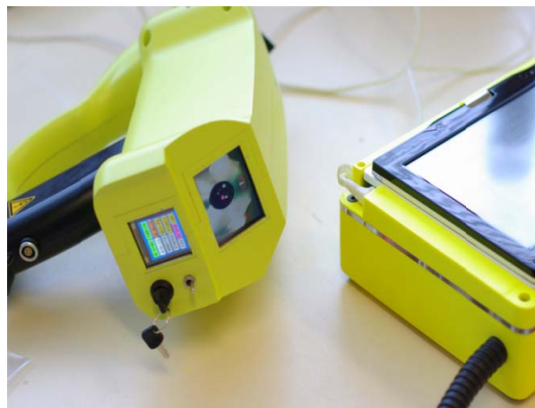
Fig. 2. Portable LIBS device used by Rakovský J. in his dissertation thesis.
