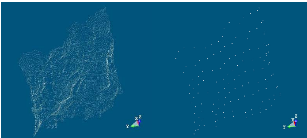
Fig. 6. Set of points of the surface No.6 with a density of 10x10 cm and 100x100 cm [3].
