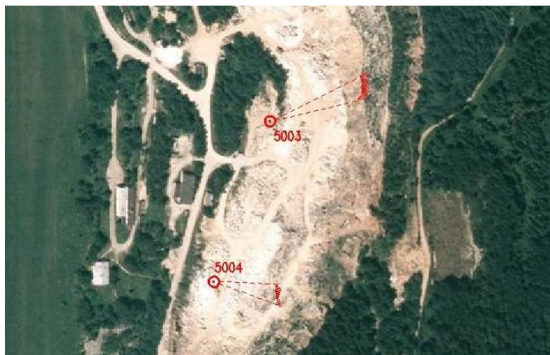
Fig. 3. Positions of the instrument survey stations at the Spišské Podhradie quarry.
