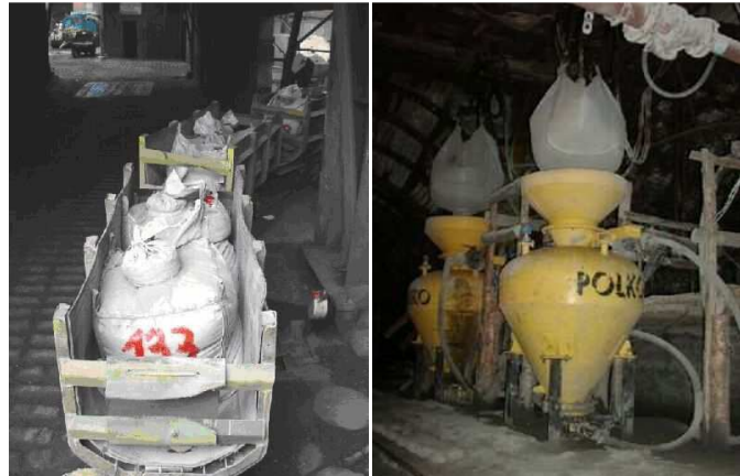
Photo 2a,b. Wheeled transport of binder from the surface in “big-bags” and its loading into chamber containers in “Anna” and “Piastr” coal mines (Madaj et al., 2002).
