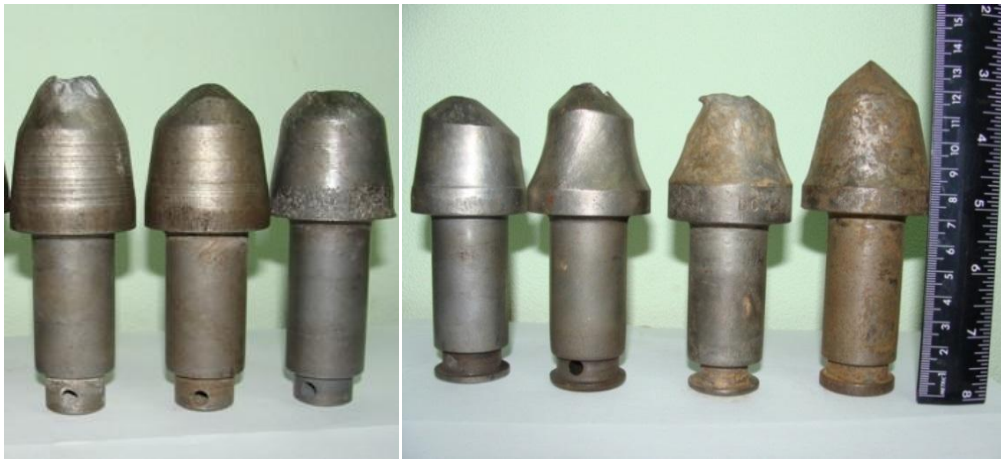
Fig. 3. Wasted mining cutters after rock breaking in the Kuzbass mines.
