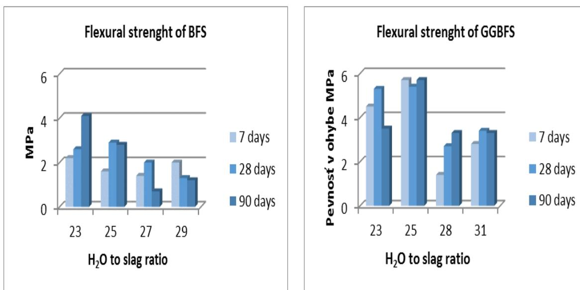
Fig. 7. Flexural strengths of BFS and GGBFS
