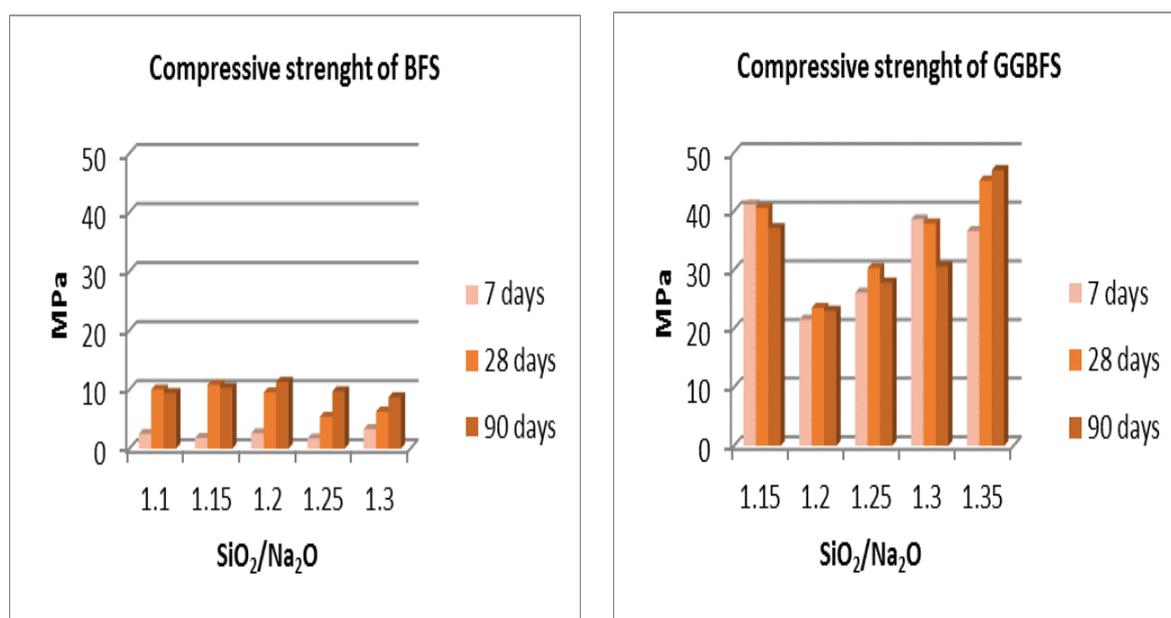
Fig. 6. Compressive strengths of BFS and GGBFS
