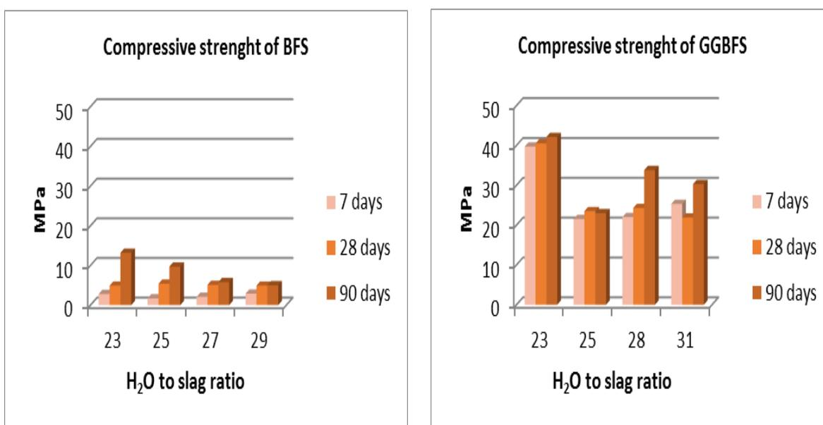
Fig. 8. Compressive strengths of BFS and GGBFS
