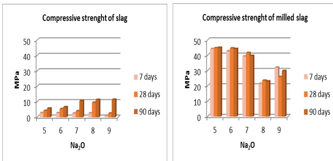
Fig. 4. Compressive strengths of BFS and GGBFS.
