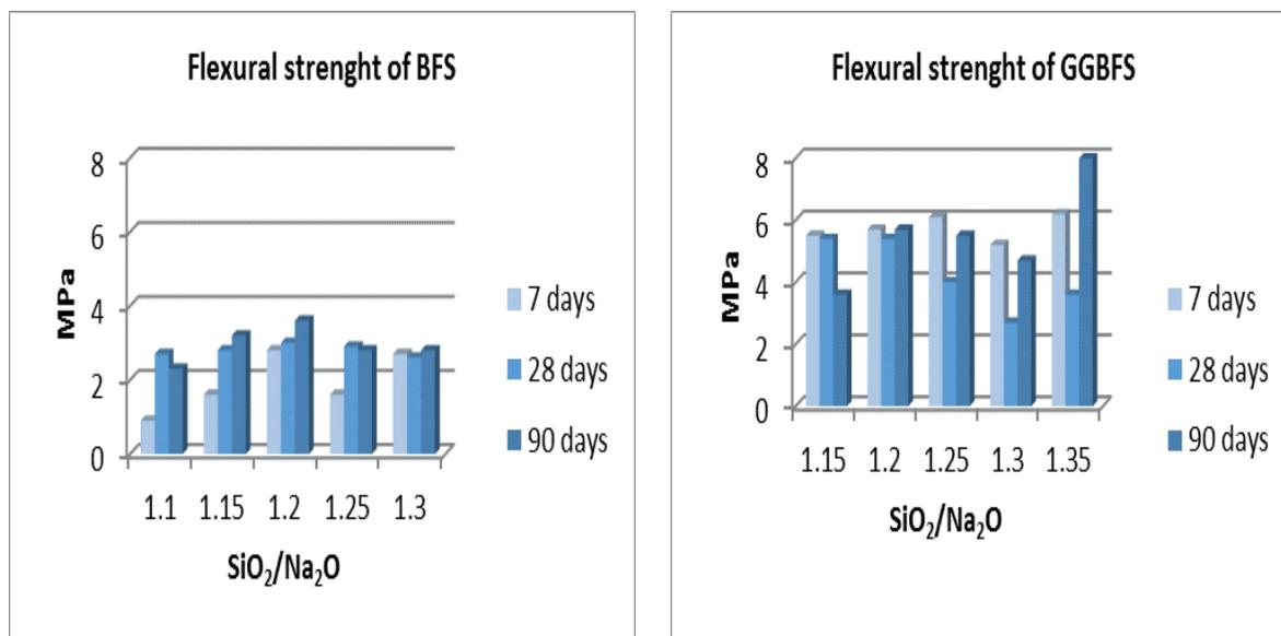
Fig. 5. Flexural strengths of BFS and GGBFS.
