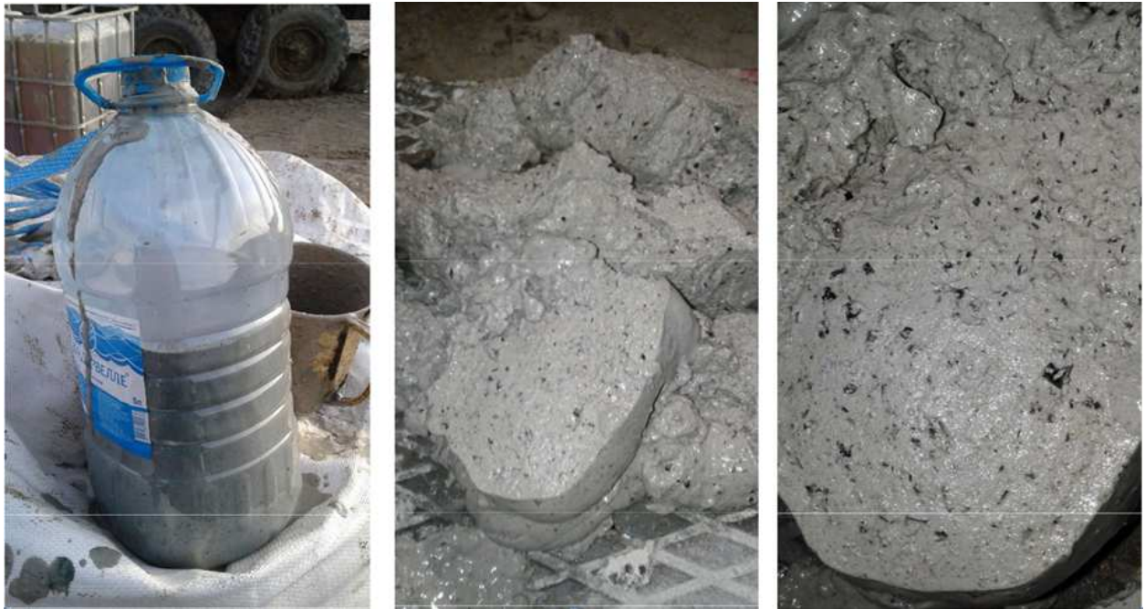
Fig.3. Sample of the insulating compound after the reaction
