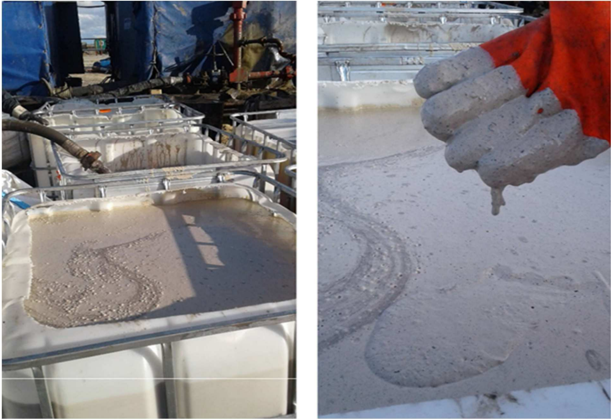
Fig. 1. Base of the insulating compound before adding chromium acetate
