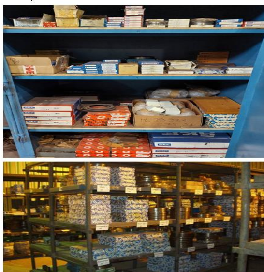
Fig. 3. 5S method for layout in the storage before and after innovation. Source: internal sources
