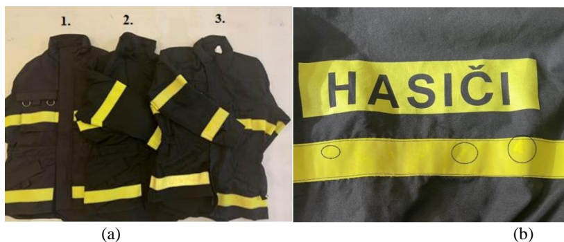
Fig. 5. Comparison of LEC samples, loss of fluorescent material (source: elaborated by authors)
