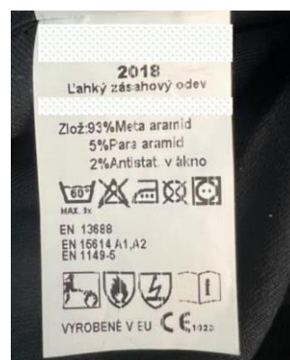
Fig. 8. A label containing not only the composition and method of maintenance but also the relevant standards (in Slovak language) (source: elaborated by authors)
