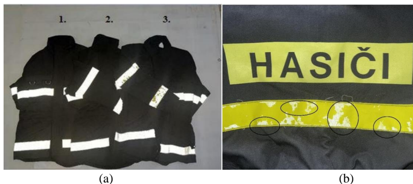
Fig. 6. Loss of fluorescent element on PPE – incoherent exposed surface (source: elaborated by authors)
