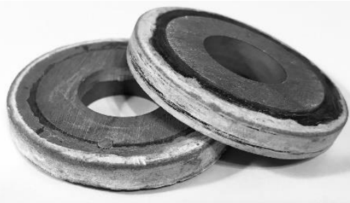
Fig. 3. Tested samples of mineraloceramic abrasive wheels.
