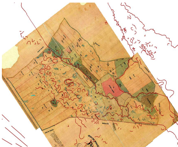
Fig. 3. The georeferenced pre-regulation map of the "Füzes-Abony area, including the Szikszó and Kisbuda farms", along with the abandoned riverbeds identified both on the satellite imagery and the archive maps (Source: Heves County Archives, Economic Archives of the Archdiocese of Eger, Manuscript Maps of Heves County).
