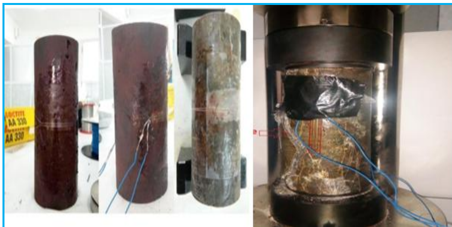
Fig. 2. Sampling and determination of the mechanical properties of the rock mass
