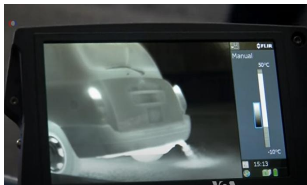
Fig. 4 Discharge of waste substances into the air - thermal image (FLIR 2019)
