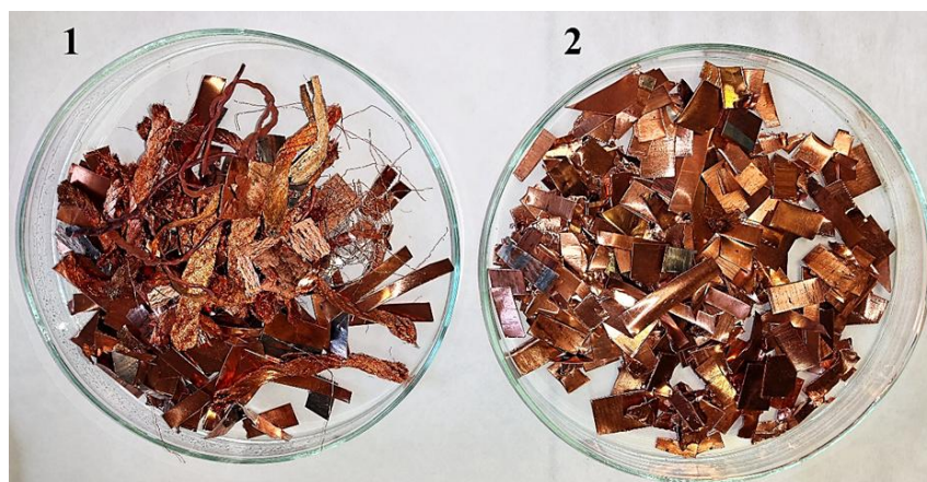
Fig. 2 Copper waste: (1) Sample 1 (leaching temperature 20 °C) and (2) Sample 2 (leaching temperature 60 °C).
