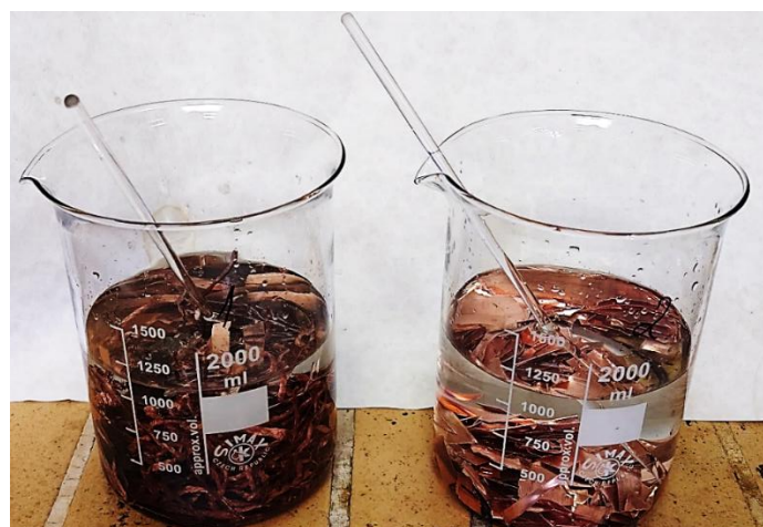
Fig. 6 Copper waste (samples 1 and 2) mixed with a leached 20% \text{H}_2\text{SO}_4 solution at the input.
