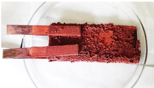
Fig. 9 Cathode surface covered with powdered copper that was expelled during electrolysis (sample 1).
