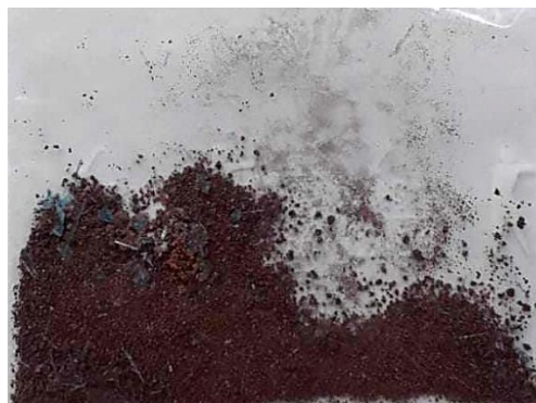
Fig. 10 Copper after electrolysis (sample 1) analysed by SEM and SEM/EDS.
