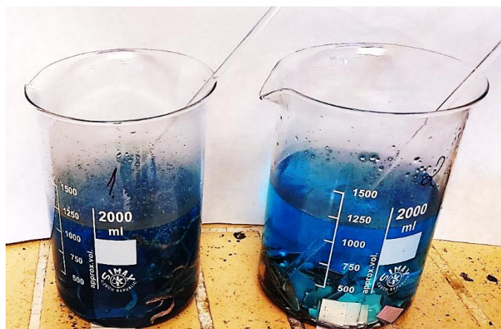
Fig. 7 Samples 1 and 2 after addition of the oxidizing agent ( \text{H}_2\text{O}_2 ).
