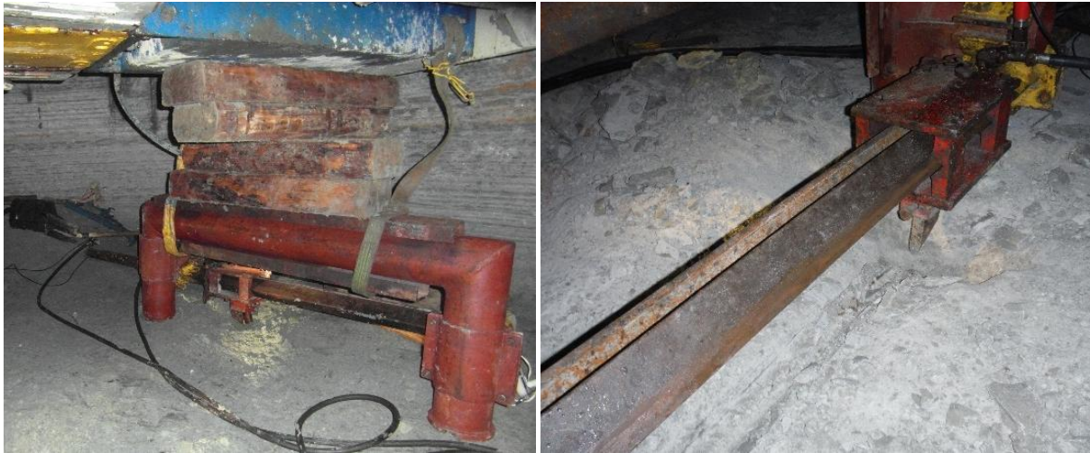
Fig. 9. Test rig prepared for workability testing in the GG-1 shaft and the cut (Boloż, 2025)
