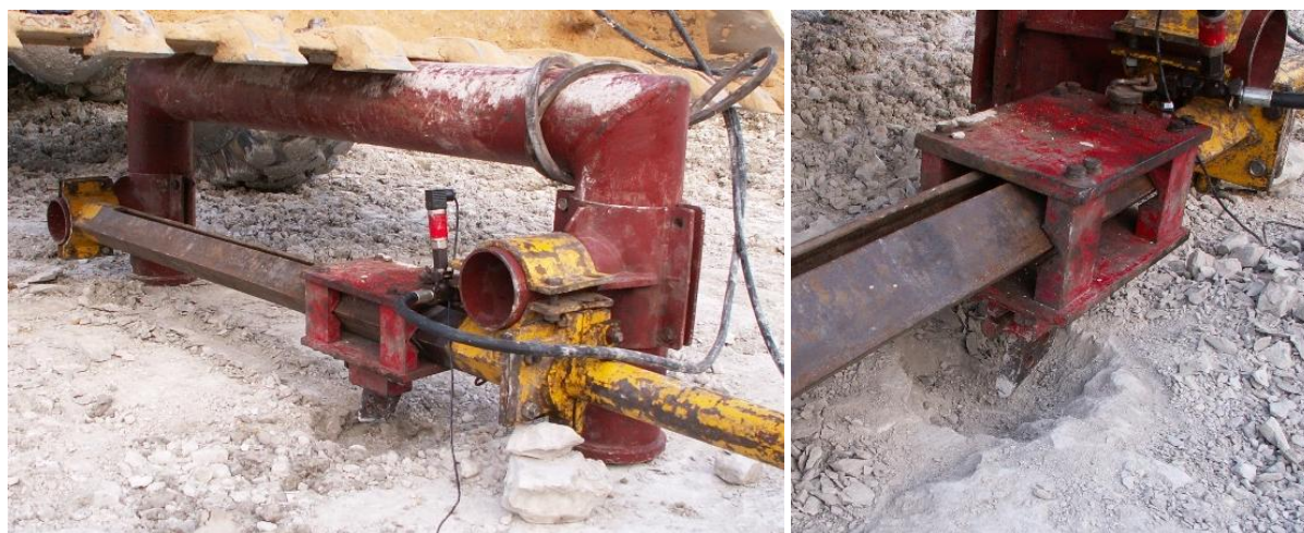
Fig. 14. Photographs of chalk marls subjected to workability tests in the mine (Bołoz, 2025)
