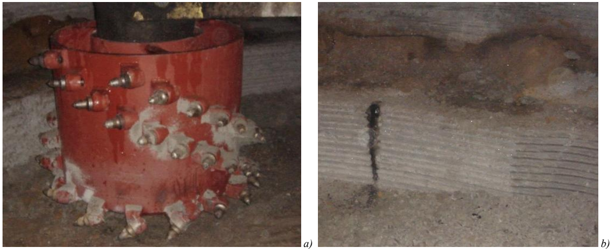
Fig. 4. Cutting head \phi 1225 \times 840 (Boloż, 2025):
