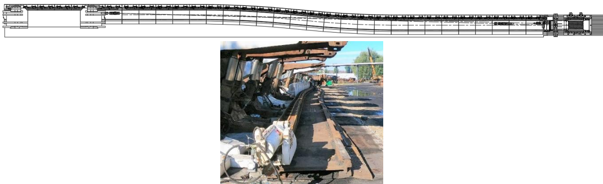
Fig. 7. Test track with a profile bent in the horizontal plane S
