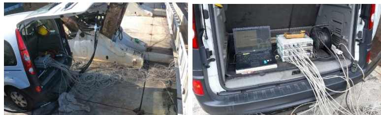
Fig. 18. Mobile measuring station enabling recording and archiving of the data during strain gauge tests.
