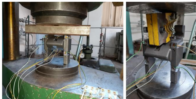
Fig. 15. Preliminary tests of toothed segments with attached strain gauges on a testing machine
