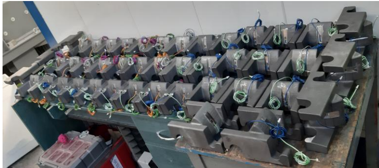
Fig. 9. Toothed segments prepared for testing with attached strain gauges and signal cables
