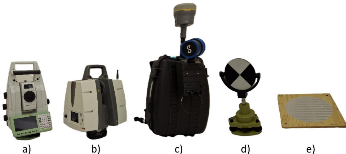
Fig. 2 Used devices and aids a) the Leica Nova TS60 robotic total station; b) the Leica ScanStation P40; c) the Emesent Hovermap ST-X with a Trimble R12i GNSS receiver mounted on a backpack; d) a black and white Leica GZT2 target on the tribrach; e) a highly reflective target for SLAM data georeferencing on the wooden desk.
