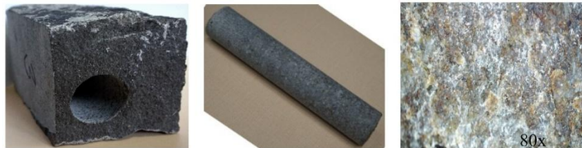
Fig. 3. Specimens of the drilled andesite (left – rock specimen, middle – drilled core, right – microscopic image of andesite surface at 80x magnification)
