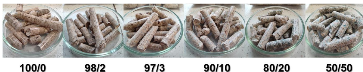
Fig. 1. Alternative fuel pellets with crushed disposable face masks and FFP2 respirators at 0%, 2%, 3%, 10%, 20%, and 50% content
